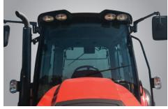
Projection Lamp Newly designed headlights allow the operator to see and work safely even in low light condition.
