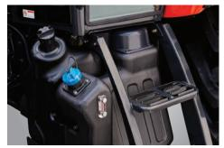
Large Fuel Tank 130 liter fuel tank provides more productive work time without the need for frequent re-fueling.
