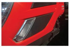
Side Working LED Lamp (Opt.) Side lights provide the operator increased visibility when turning.
