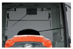
**Standard Wipers** Front and rear window wipers are positioned to minimize impact to the operator's field of vision.
