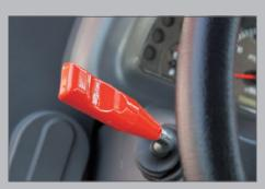
Synchronized & Power Shuttle Lever The synchronized shuttle lever makes it easy to change direction from forwards to backwards and reduces operator fatigue. The power shuttle lever provides softer shuttle operation and allows the operator to perform loader work without pressing the foot clutch pedal.
