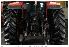
**External Hydraulic Lift Cylinder** External hydraulic lift cylinders increases the lift capacity up to 3,630kgf (610mm from the lifting point).
