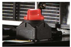
**Battery Disconnect Switch** Standard on PX Series tractors, the battery disconnect switch can help improve battery life when storing for large amounts of time.
