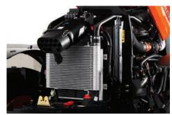
**Turbocharged, Intercooled Engine** The turbocharged engine with Air to Air Intercooler ensures the PX Series has the power the operator needs. The dual air cleaner offers increased filtration which extends the filter life.
