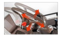
Tilting and telescopic steering wheel adjustable to be proper to driver. (tilting 24degree, telescopic length 50mm)
