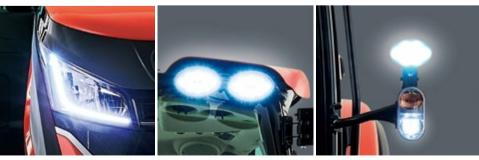
Full LED Lamps and Front/Rear Working Lights (LED option)
